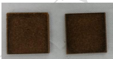
Figure 1: Thermopressed agricultural material in sheet form
