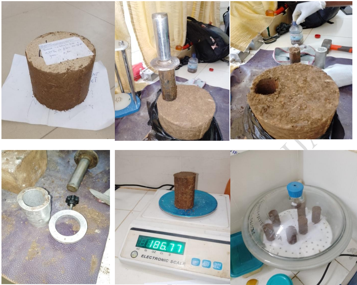
Figure 6. Specimen preparation steps.
