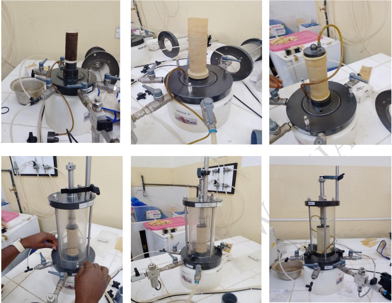
Figure 7. Triaxial tests on specimens.
