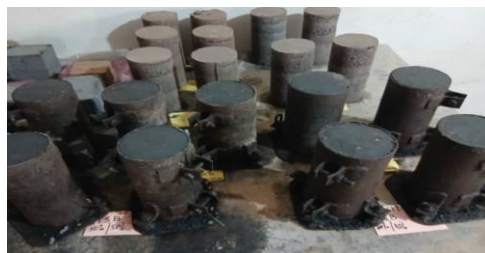
92 93 Figure 2: Test specimens of the various mixtures studied
