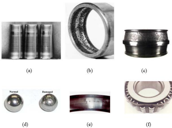
Figure 5. (a) Wear of rolling elements (b) Corrosion of the outer ring (c) Friction of the rolling surface (Hamouche, 2022) (d) Defect on a ball (e) Spalling of the inner ring (e) Spalling of the outer ring (f) Deformation of the cage (HOTAIT, 2020)
