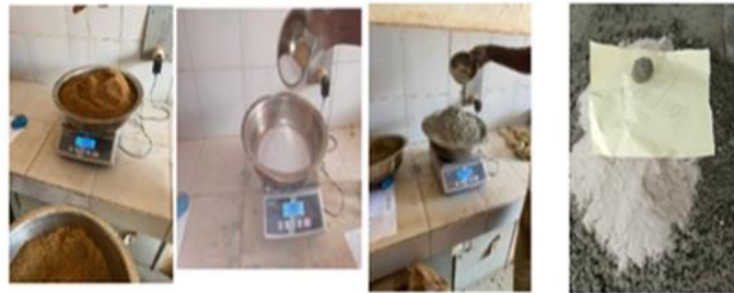
Figure 3.b: Weighing crushed sand, glass powder and cement using an electronic balance
