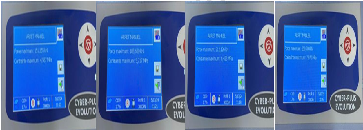
Figure 8: Stresses and fracture loads of the specimens
