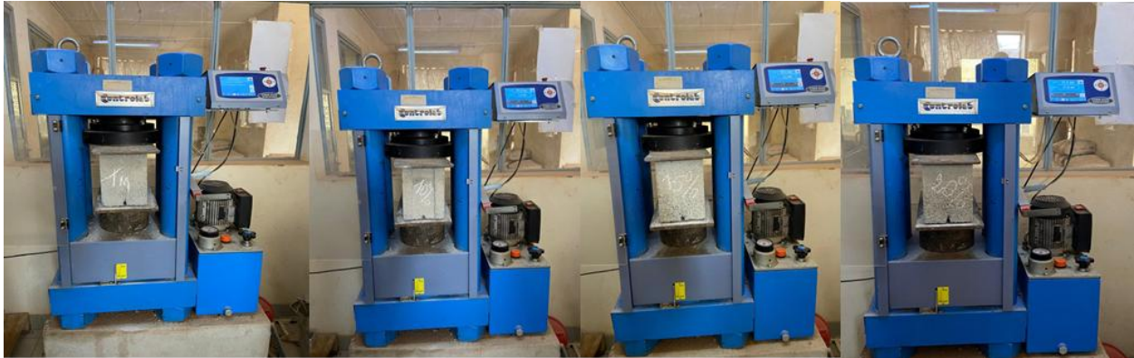
Figure 7: Crushing of concrete block samples in the hydraulic press
