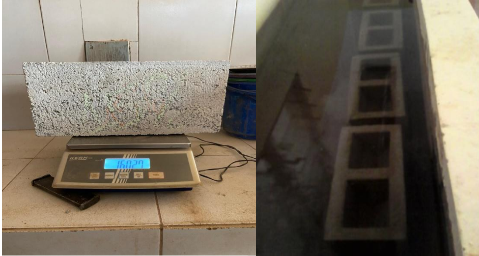
Figure 10: Weighing the concrete block before submerging it in the water-filled tank
