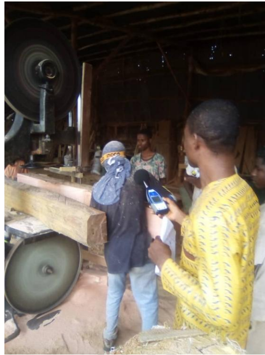
Photo 7: Measurement of equivalent continuous sound pressure levels L_{p,A,eqT}
