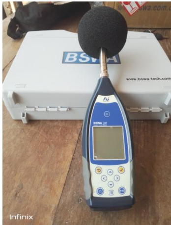
88 Photo 5: Integrating sound level meter BSWA 308, class 1, accuracy 0.7
