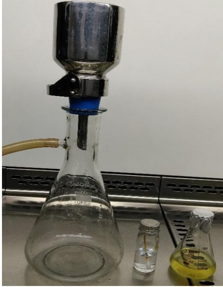
114 Fig.2: Filter Assembly,Swab sample and Buffered Peptone water,
